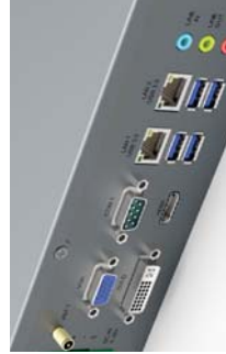
Side B - Huge I/F capability towards the field, 3 display ports , 4 USB 3.0 , 2 independent LAN ports.
